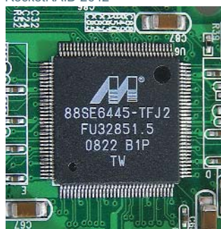
■ Chip Marvell88SE6445 for four ports Serial Attached SCSI on bus PCI- Express x4.
